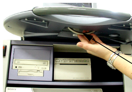
Figure 4-29 Locking Lever under Control Console
