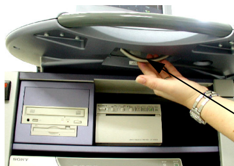
Figure 5-22 Locking Bolt under Control Console
