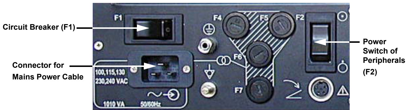
Figure 3-8 Circuit Breaker (F1) and Power Switch of Peripherals (F2)
