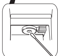
Cap pierce nozzle (bottom view seen from the front panel side with the tube holder opened)
