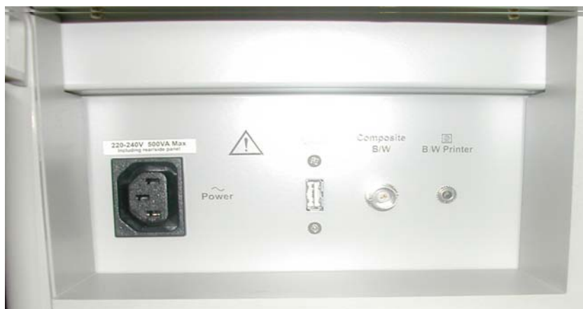
Figure 8-241 USB Port - OP Printer Bracket Back Panel
