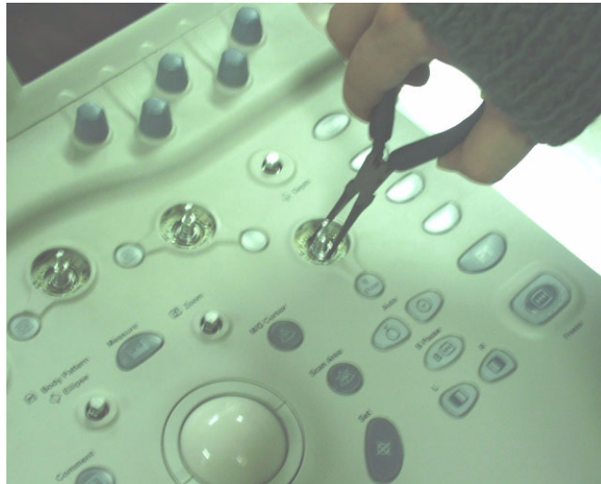
Figure 8-28 Pulling Out encoder nuts
