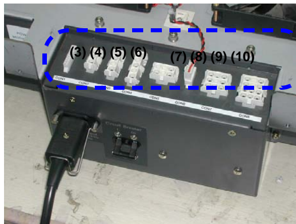
Figure 8-183 Disconnecting 8 connectors
