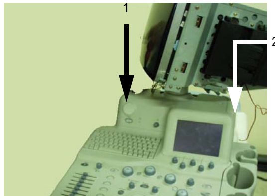
Figure 8-18 Unscrew two screws on the shoulder
