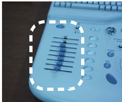
Figure 8-30 Removing TGC Knobs
