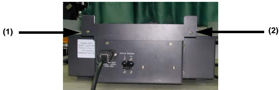
Figure 8-182 Removing the Rear Connector Bracket
