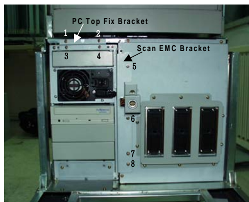
Figure 8-169 ATX SMPS Replacement
