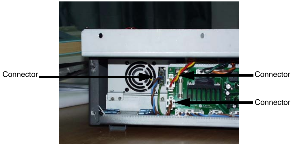
Figure 6-1 Disconnect 3 connectors
