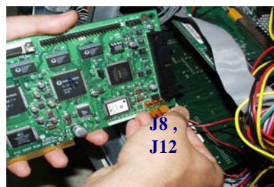
Figure 8-163 Disconnect 2 connectors
