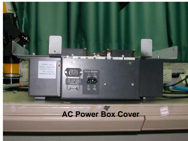
Figure 8-193 Unscrew 6 screws to remove AC Power Box
