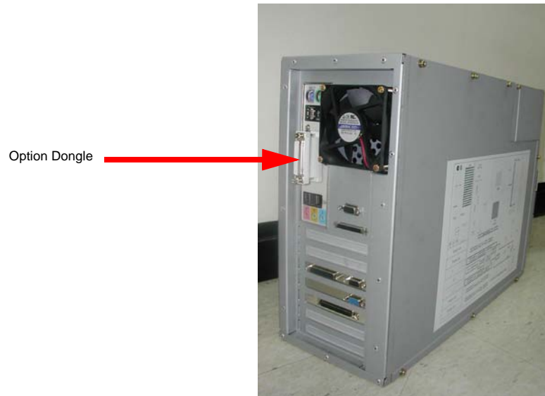
Figure 8-101 BT05 BEP3 Option Dongle replacement
