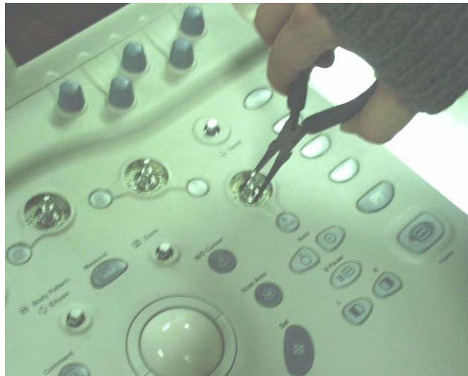
Figure 8-56 Pulling Out encoder nuts
