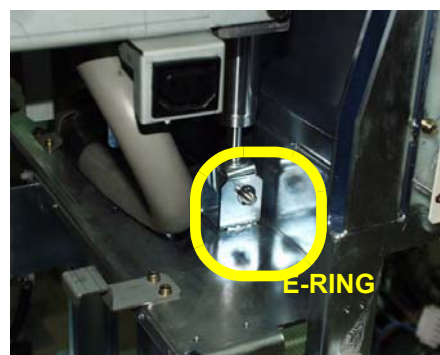
Figure 8-107 Remove E-Ring
