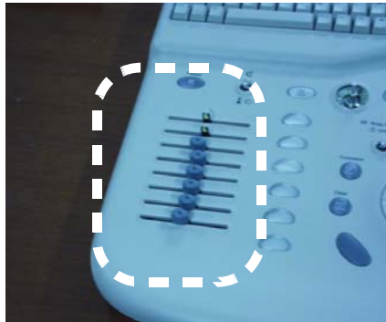
Figure 8-60 Removing TGC Knobs
