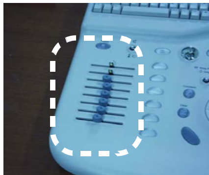
Figure 8-58 Removing TGC Knobs
